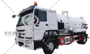
HOWO Sewage Suction Truck Driving Type: 4x2 Engine Power: 300-340hp Tank Capacity: 12m 3
