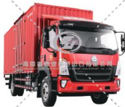
HOWO Light Van Truck Driving Type: 4x2 Engine Power: 110-160hp Van size: 4800*2200*2050mm
